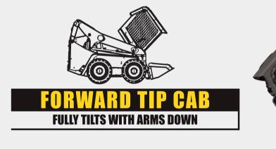
The only cab that fully tips forward with the arms down, providing complete access to all maintenance components, no matter what the situation.
