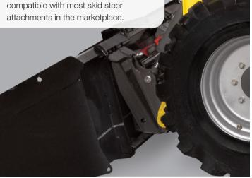
Hydraulic Universal Attachment Plate (optional on all machines) allows the operator to quickly and easily install and remove attachments without ever leaving the cab. (Only leave if auxiliary hydraulic connections are required).
